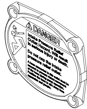
RELIEF VALVE OUTLET WARNING PLATE
