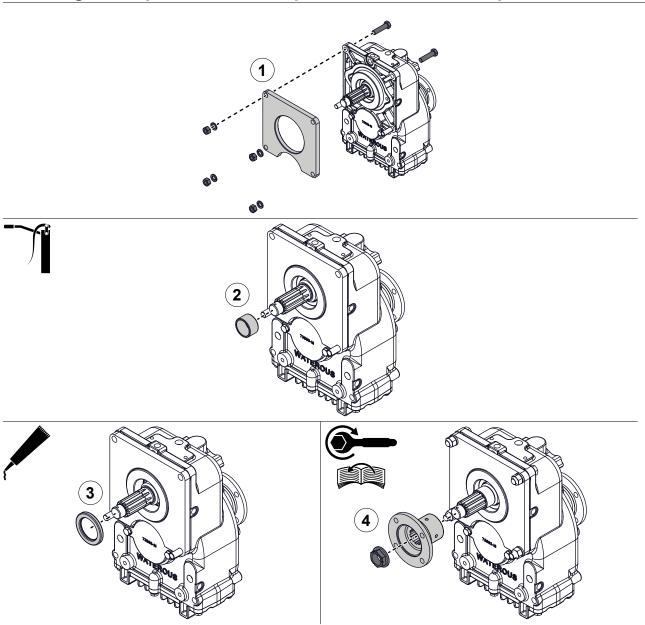
Use the illustrations and instructions to install the impeller-shaft components.
