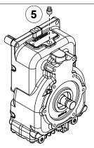
Use the illustrations and instructions to add oil to the power take-off. The illustrations may not represent your specific power take-off orientation. Refer to the SPL for your application to locate the oil-fill and oil level plug for your orientation. Refer to the documentation provided with your equipment to determine the type of lubricant, and
