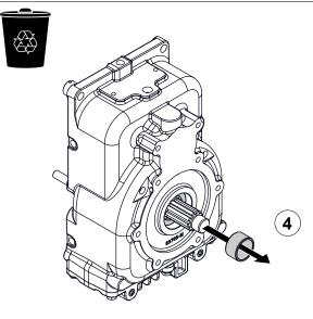
Use the illustrations and instructions to remove the PTO adapters and plate.
