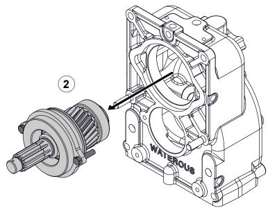
Use the illustrations and instructions to remove the bearing housing.
