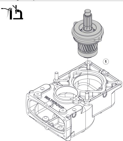
Use the illustration and instruction to install the impeller-shaft assembly.
