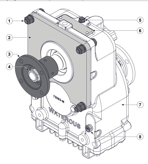
Use the illustration to identify various components on the power take-off (PTO).
