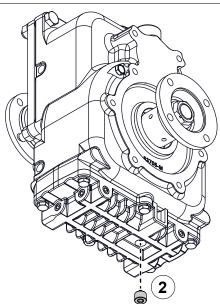
Use the illustrations and instructions to drain the oil from the power take-off. The illustrations may not represent your specific power take-off orientation. Refer to the SPL for your application to locate the oil-drain plug for your orientation.
