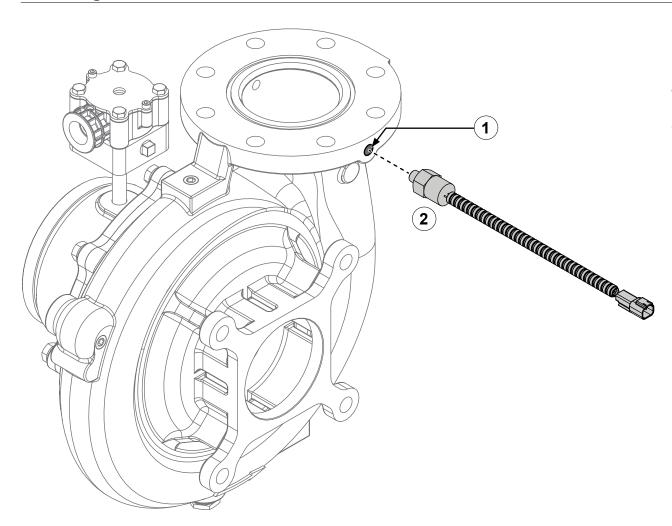
Use the illustration and instructions to install the pressure switch. The pressure switch is only required when operating the pump in auto-prime mode.
