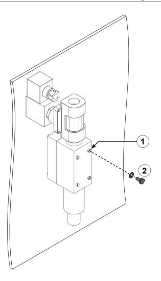
The air primer is typically factory-mounted on the transmission, but it can also be mounted remotely. Use the illustration and instructions to install the air primer. Before you install the air primer, refer to: "Installation Requirements" on page 33 to determine a proper install location and orientation.
