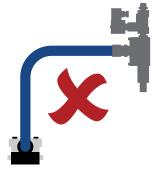
Only install the air primer with the exhaust directed downward.
