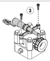
Use the illustration and instructions to install the optional priming valve solenoid.
