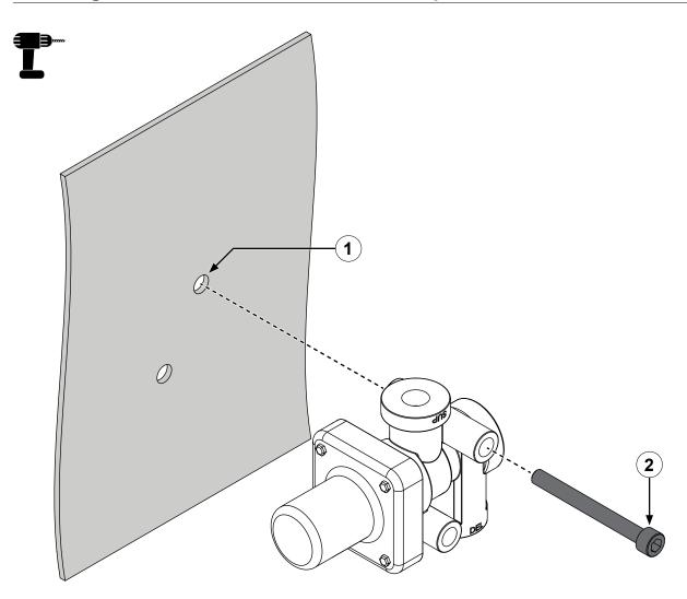
Use the illustration and instructions to install the pressure protection switch.
