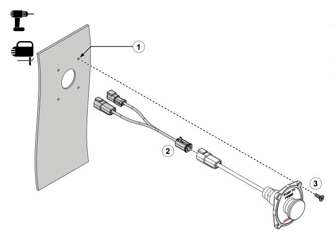
Use the illustration and instructions to mount the oversized push button switch on the panel.
