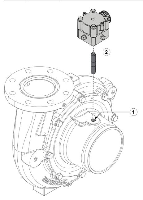
Use the illustration and instructions to install the priming valve. Use appropriate locally sourced air line and fittings. The illustration shows a typical priming valve installation on a typical fire pump—your specific application my differ in appearance. Regardless of appearance, use the following guidelines to install the priming valve in your application:
