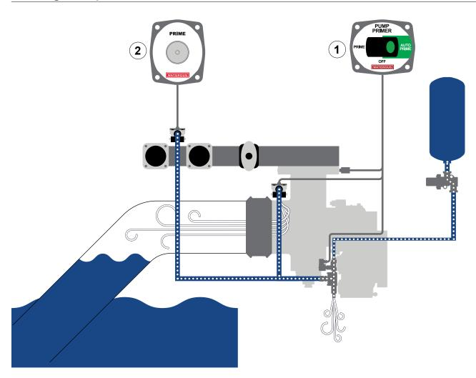
Use the illustration and instructions to prime an application with multiple priming valves. Know that each priming valve should be isolated and operated independently.
