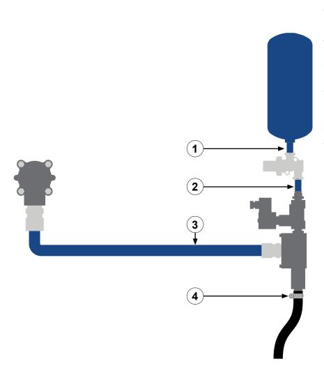
Use the illustration and instructions to connect the vacuum components. Your application may include factory-installed connected components. Otherwise, follow the applicable instructions to connect the components in your application. Use appropriate locally sourced air line and fittings.
