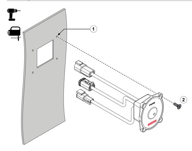
Use the illustration and instructions to mount the standard push button switch on the panel.
