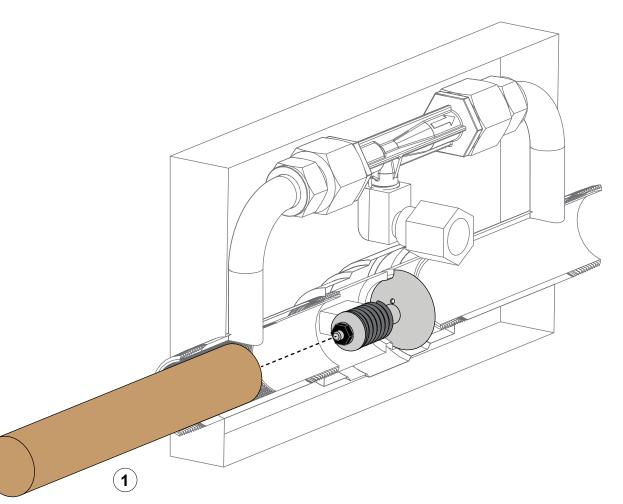
Use the illustration and instructions to clear a check valve jam condition if a jam condition occurs.
