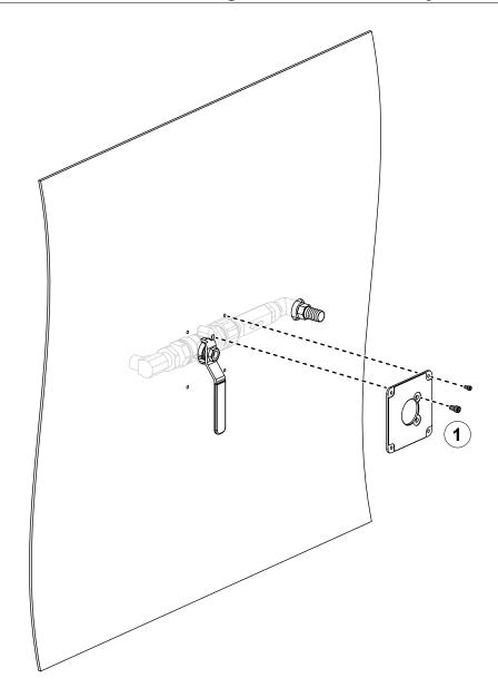
Use the illustration and instructions to remotely mount the eductor and panel mount the valve assembly.
