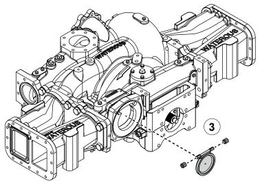
Use the illustrations and instructions to remove the tank intake adapter.
