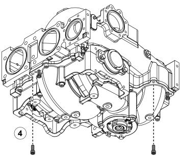
Use the illustrations and instructions to disassemble the pump body.
