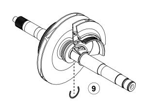
Use the illustrations and instructions to disassemble the impeller shaft.
