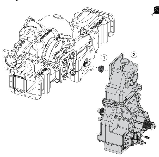
Use the illustration and instructions to install the transmission onto the pump—C22 transmission shown.
