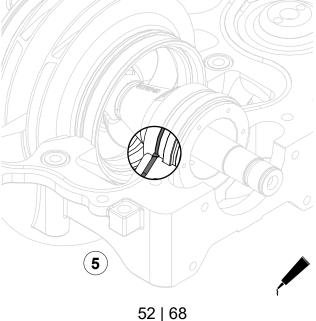
Use the illustrations and instructions to install the impeller shaft assembly into the volute cover.
