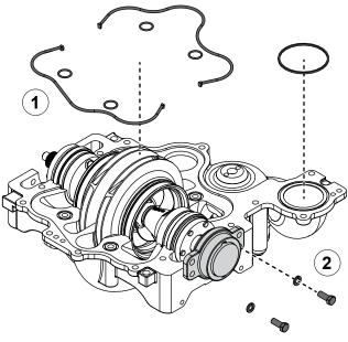
Use the illustrations and instructions to remove the impeller shaft assembly from the volute cover.
