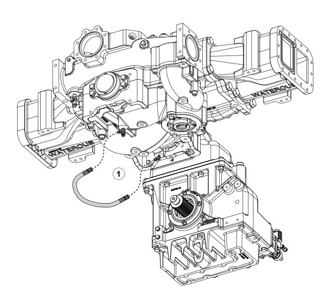
Use the illustration and instructions to remove the seal cooling hose.
