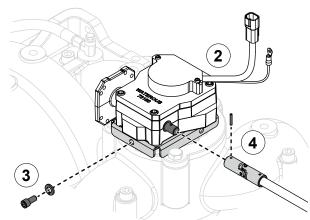
Use the illustration and instructions to install the bottom-mounted transfer valve actuator—manual option shown.
