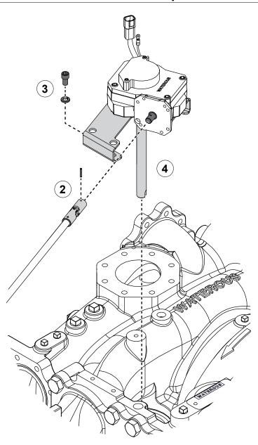
Use the illustration and instructions to remove the top-mounted transfer valve actuator—manual option shown.
