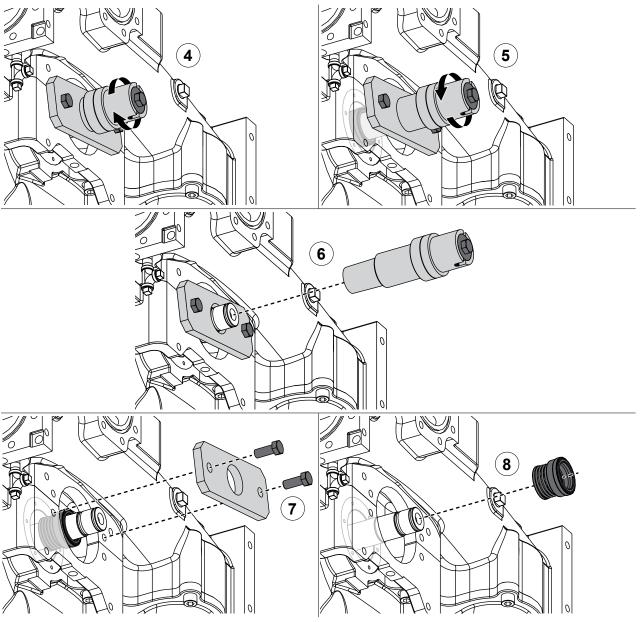
Use the illustrations and instructions to remove the mechanical seal without disassembling the pump. The tools being used are included in the Mechanical Seal Removal and Installation Kit (K 628).
