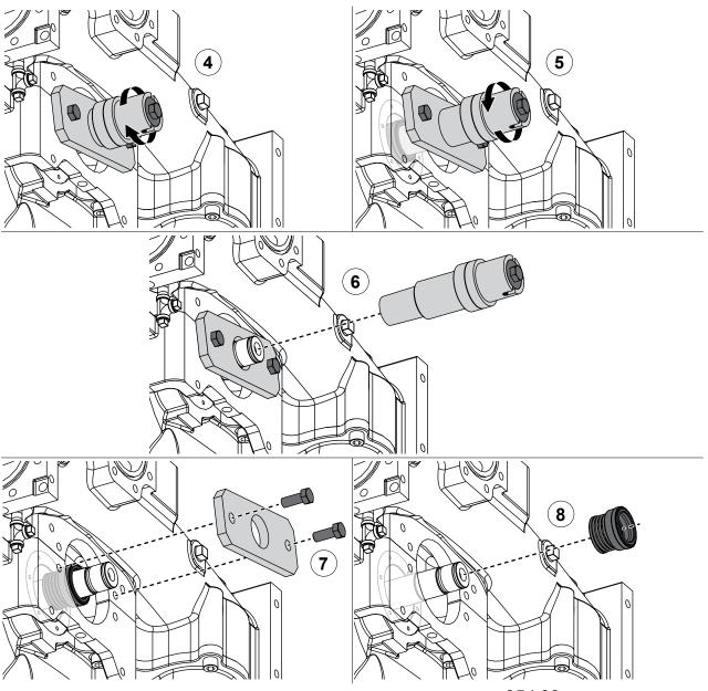
Use the illustrations and instructions to remove the mechanical seal without disassembling the pump. The tools being used are included in the Mechanical Seal Removal and Installation Kit (K 628).
