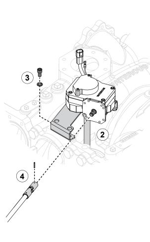
Use the illustration and instructions to install the top-mounted transfer valve actuator—manual option shown.
