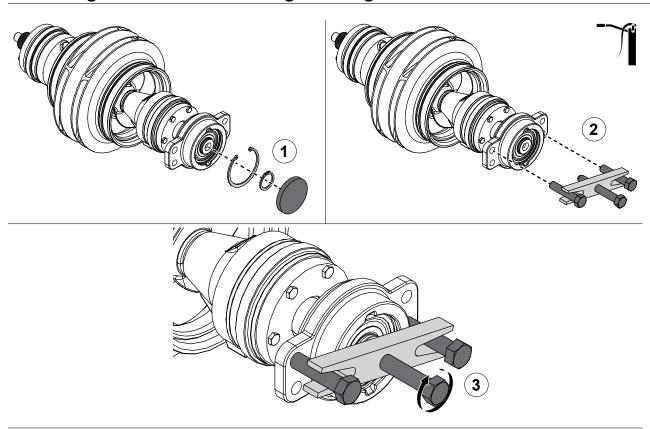
Use the illustrations and instructions to remove the outboard bearing housing. The tools being used are included in the Outboard Bearing Removal and Installation Kit (K 956).
