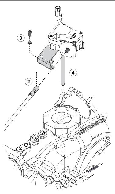
Use the illustration and instructions to remove the top-mounted transfer valve actuator—manual option shown.
