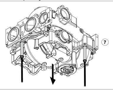
Use the illustrations and instructions to disassemble the pump body.
