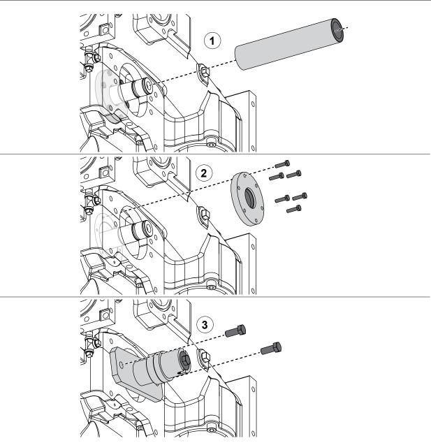
Use the illustrations and instructions to remove the mechanical seal without disassembling the pump. The tools being used are included in the Mechanical Seal Removal and Installation Kit (K 628).
