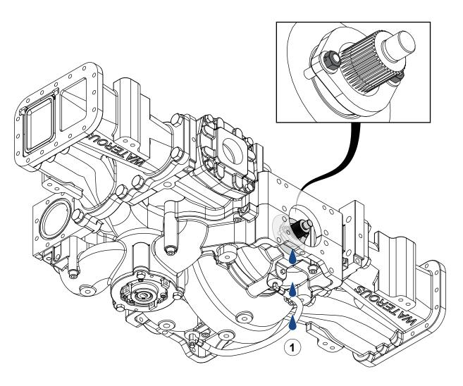
Use the illustration and instructions to adjust the packing glands after installing the pump into the apparatus. Do not calculate the drip rate until the leakage runs clear.
