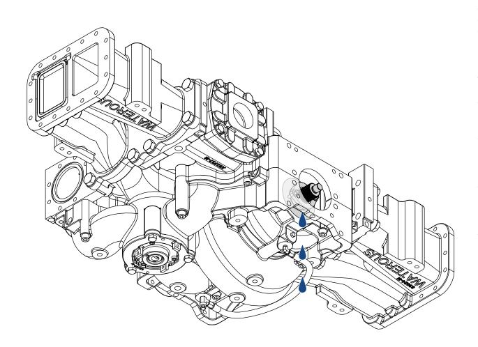
If your configuration includes an impeller shaft with packing, use the illustration and instructions to adjust the packing after installing the pump into the apparatus.
