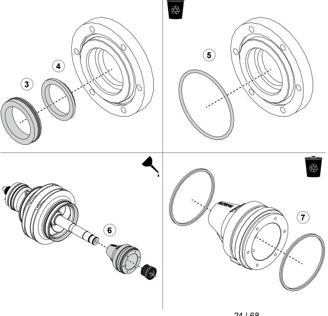
Use the illustrations and instructions to disassemble the impeller shaft.
