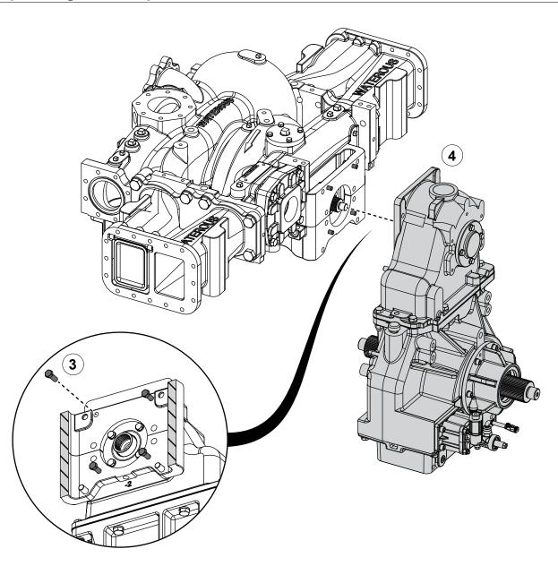
Use the illustration and instructions to separate the pump and transmission.
