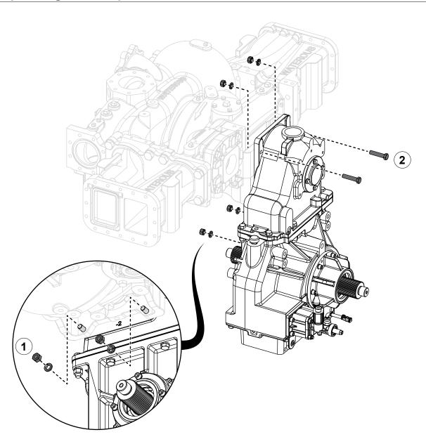
Use the illustration and instructions to separate the pump and transmission—C22 transmission shown.
