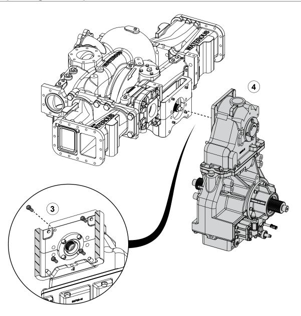
Use the illustration and instructions to separate the pump and transmission.
