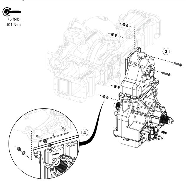
Use the illustration and instructions to install the transmission onto the pump.
