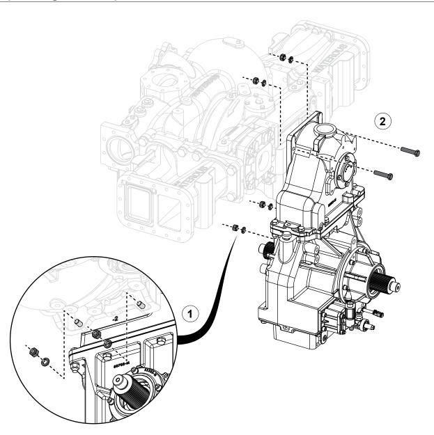
Use the illustration and instructions to separate the pump and transmission—C22 transmission shown.
