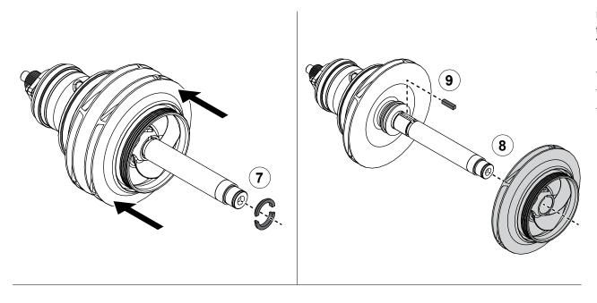
Use the illustrations and instructions to disassemble the impeller shaft.
