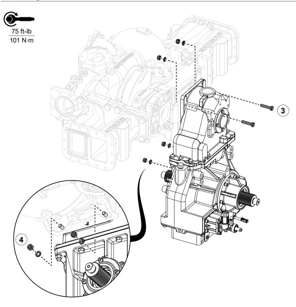
Use the illustration and instructions to install the transmission onto the pump.
