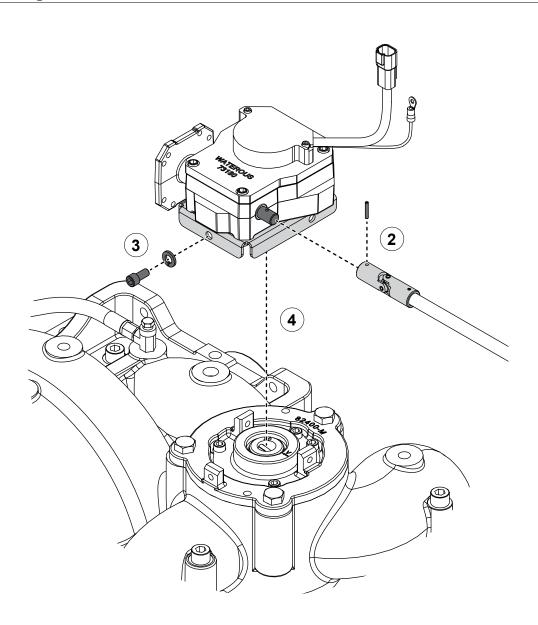
Use the illustration and instructions to remove the bottom-mounted transfer valve actuator—manual option shown.
