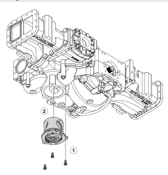
Use the illustration and instructions to remove the transfer valve from the pump.
