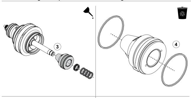
Use the illustrations and instructions to disassemble the impeller shaft.
