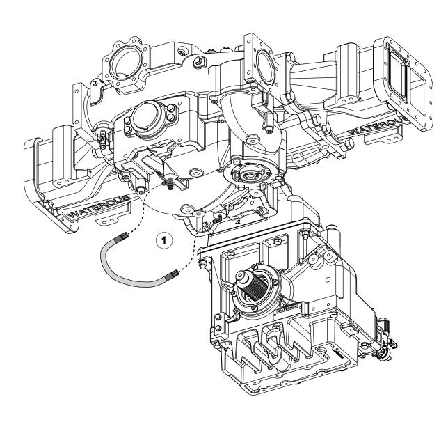
Use the illustration and instructions to install the seal cooling hose.
