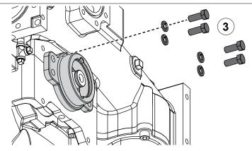
Use the illustrations and instructions to install the outboard bearing housing.
