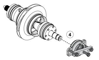
Use the illustrations and instructions to remove the outboard bearing housing. The tools being used are included in the Outboard Bearing Removal and Installation Kit (K 956).
