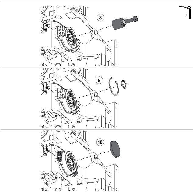
Use the illustrations and instructions to install the outboard bearing housing. The tools being used are included in the Outboard Bearing Removal and Installation Kit (K 956).
