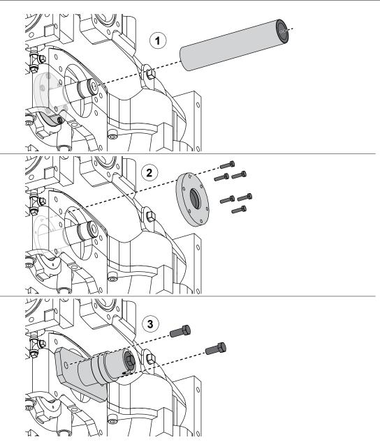
Use the illustrations and instructions to remove the mechanical seal without disassembling the pump. The tools being used are included in the Mechanical Seal Removal and Installation Kit (K 628).
