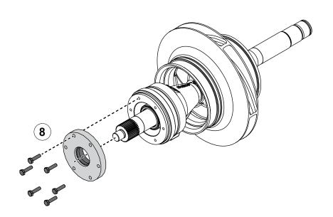
Use the illustrations and instructions to disassemble the impeller shaft.
