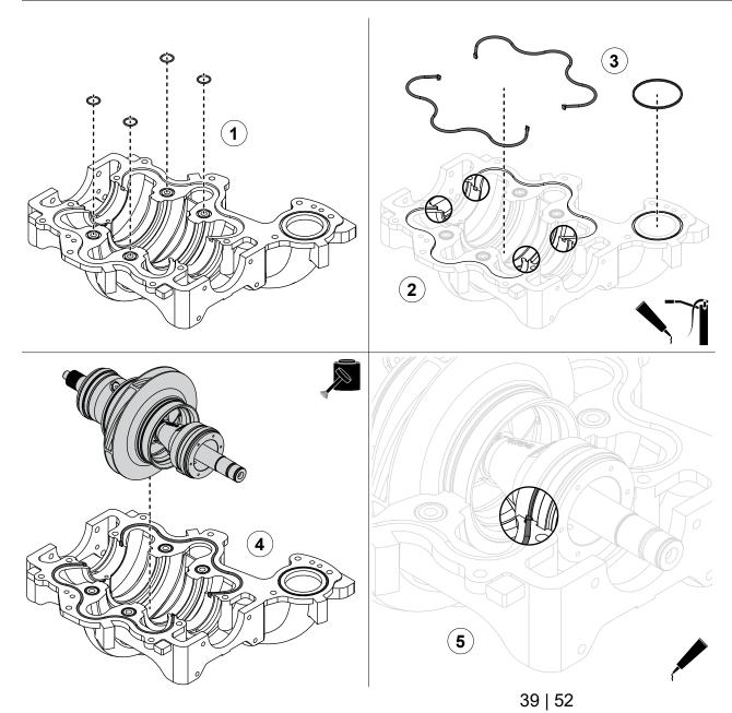
Use the illustrations and instructions to install the impeller shaft assembly into the volute cover.
