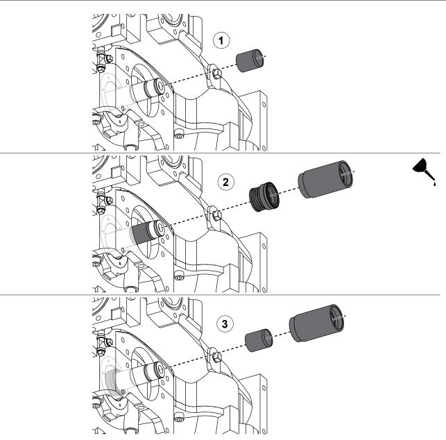
Use the illustrations and instructions to install the mechanical seals. The tools being used are included in the Mechanical Seal Removal and Installation Kit (K 628).
