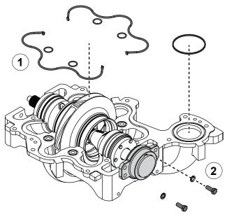
Use the illustrations and instructions to remove the impeller shaft assembly from the volute cover.
