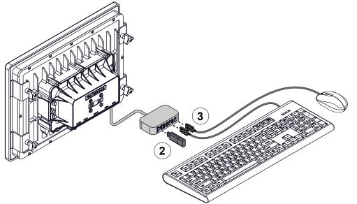
Use the illustrations and instructions to connect an external keyboard and USB drive to the control panel. The USB drive can be used to download and save the current configuration file, upload a new configuration, or restore a previous configuration.
