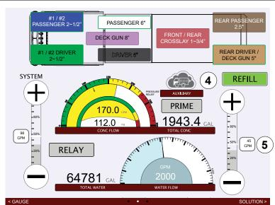
Use the illustrations and instructions to refill the on-board concentrate supply tank from an auxiliary source. This is useful when manually refilling the on-board supply tank is not practical. Refilling the on-board supply tank can take place concurrently with normal discharge operations.
