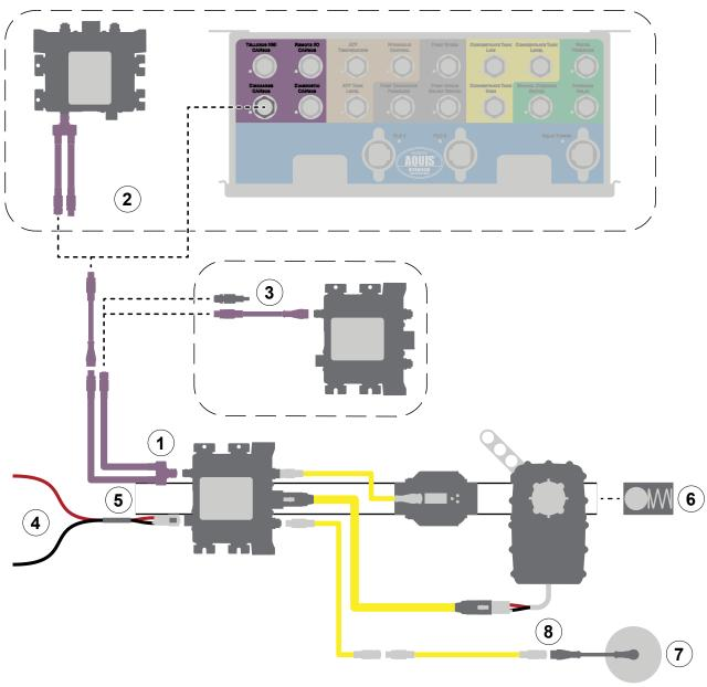
Use the illustration and instructions to install the 2-inch DLA. To connect to the apparatus plumbing, refer to: "Plumbing Layout" on page 36.
