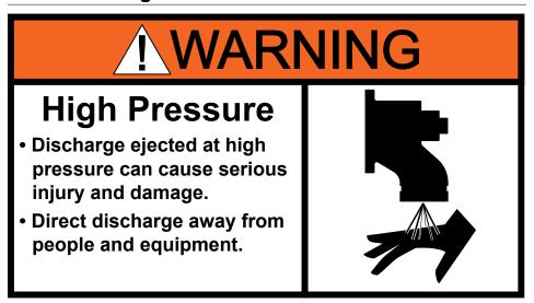
An over-pressure event is an event that causes concentrate to discharge into the on-board tank or external reservoir at a high pressure. Typically two conditions cause over-pressure events: the pressure relief valve is activated or you manually over-prime the system.
