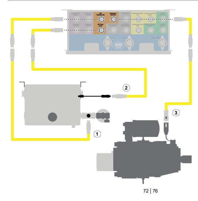
Use the illustration and instructions to connect the hydraulic sensors and hydraulic pump to the control box.
