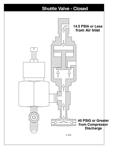
When the compressor is running, the CIAP is always 14.5 psia or less and the CDAP is 40 psig or greater (minimum pressure valve setting), allowing the shuttle valve to stay closed.
