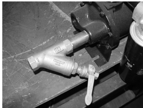
Figure 4 Wye-strainer installed, with cleanout valve.
