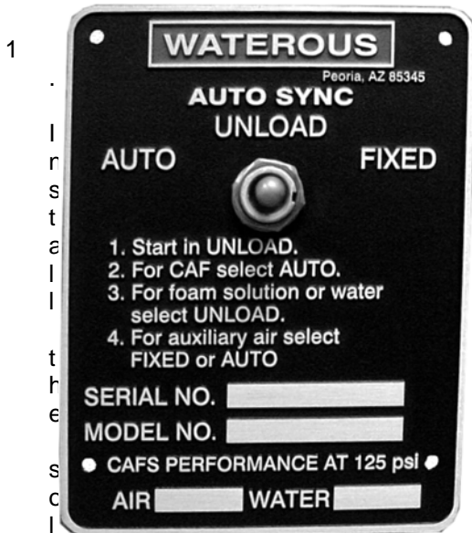
Electrical Auto Sync Control Switch
