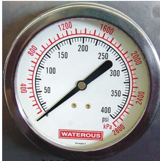
Figure 21 Typical Air Pressure Gauge
