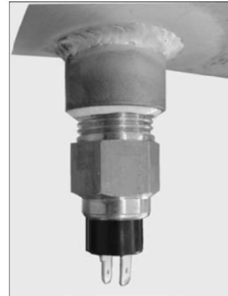
Temperature sender on Sump
