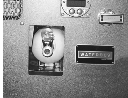
Ideal installation, with sight glass and oil fill easy to access
