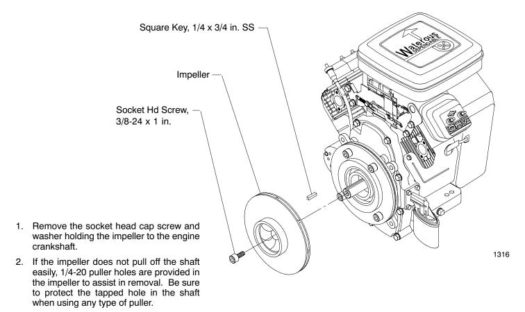
3. Remove the impeller key.
