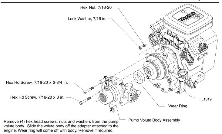
The muffler and control panel are shown removed for clarity.
