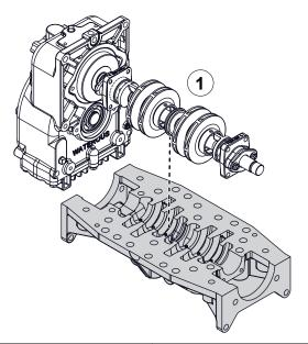
Use the illustrations and instructions to secure the lower pump body to the transmission case.
