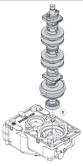
Use the illustrations and instructions to install the impeller shaft assembly.
