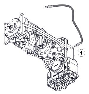
Use the illustrations and instructions to install the packing cooler hose. Insert one end of the hose into the pump
