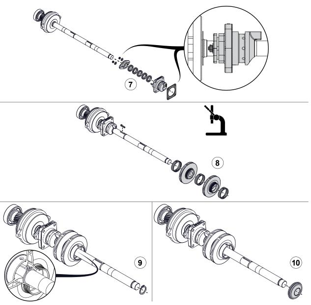
Use the illustrations and instructions to assemble the impeller shaft.
