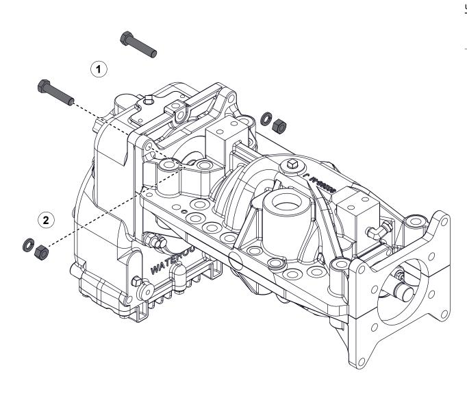
Use the illustration and instructions to install the upper transmission mounting hardware.
