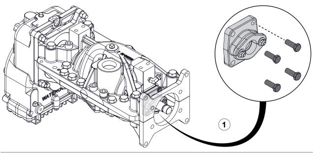
Use the illustrations and instructions to install the packing housing hardware.
