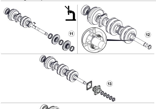
Use the illustrations and instructions to assemble the impeller shaft.
