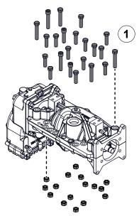
Use the illustrations and instructions to install the upper and lower pump body hardware.
