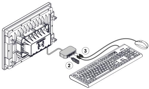
Use the illustrations and instructions to connect an external keyboard and USB drive to the control panel. The USB drive can be used to download and save the current configuration file, upload a new configuration, or restore a previous configuration.
