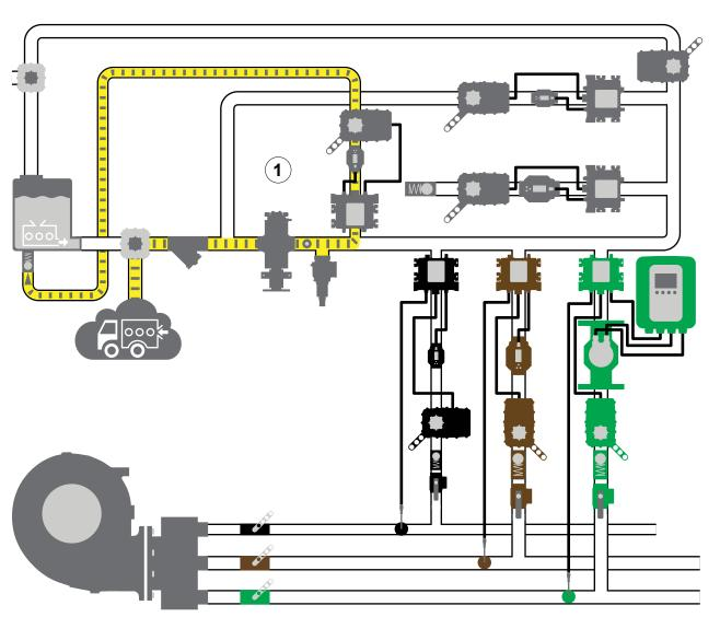
Use the illustration and instructions to understand the system activity when you refill the on-board concentrate supply tank. You can operate the discharges while refilling the tank.
