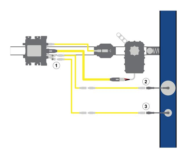
Use the illustration and instructions to install the Y-splitter when measuring the discharge pressure at the solution-capable discharge.
