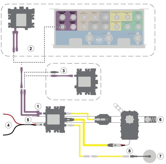
Use the illustration and instructions to install the 1-inch DLA. To connect to the apparatus plumbing, refer to: "Plumbing Layout" on page 36.
