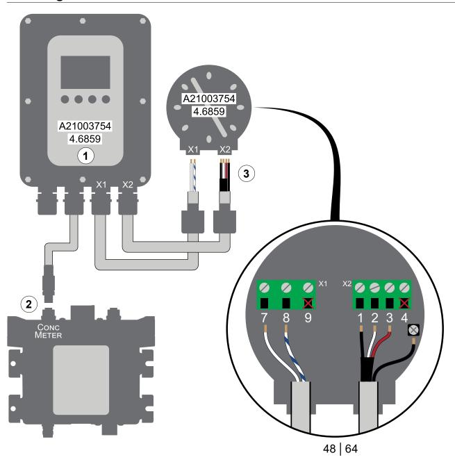
Use the illustration and instructions to install the transmitter and flowmeter. To connect the flowmeter to the apparatus plumbing, refer to: "Plumbing Layout" on page 36. Mount the transmitter close to the DLA and make sure that it is accessible for setup and maintenance. The transmitter is wired at the factory and only requires the wire leads to be connected to the flowmeter.
