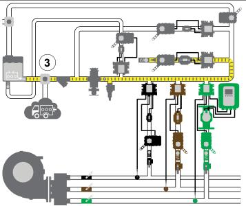
Use the illustrations and instructions to transfer concentrate to another location. If included in your application, you can use the transfer line to move the concentrate from the on-board tank or external source to another location. You can operate the discharges while transferring concentrate.
