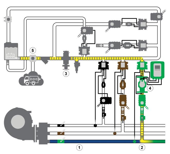
Use the illustration and instructions to understand the system activity when you enable a DLA. Remember that an enabled DLA is only active when the associated line is flowing water.
