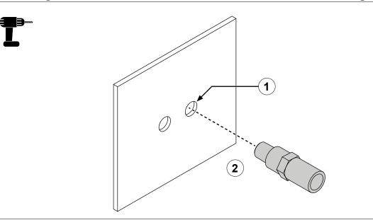
Use the illustration and instructions to install the thermal valve and switch into the piping when no discharge fittings are available.
