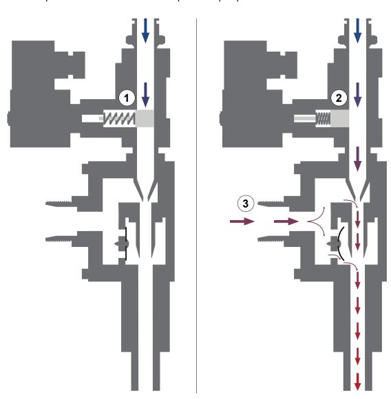
Use the illustration and instruction to understand the principles of operation of the air primer.
