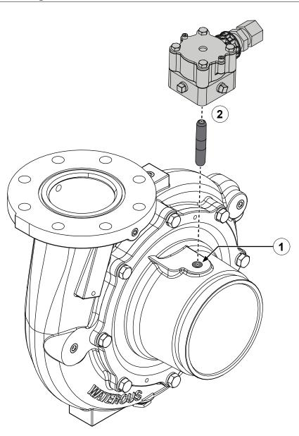
Use the illustration and instructions to install the priming valve. The illustration shows a typical priming valve installation on a typical fire pump—your specific application my differ in appearance. Regardless of appearance, use the following guidelines to install the priming valve in your application:
