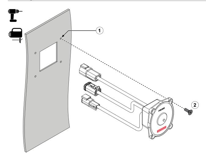
Use the illustration and instructions to mount the manual-prime switch on the panel.
