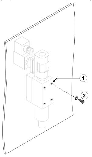
Use the illustration and instruction to install the air primer. Before you install the air primer, refer to: "Installation Requirements" on page 27 to determine a proper install location and orientation.
