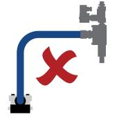
Only install the air primer with the exhaust directed downward.
