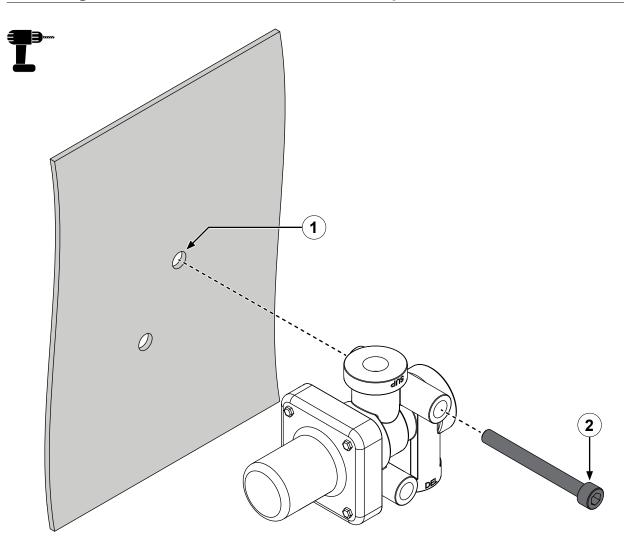
Use the illustration and instructions to install the pressure protection switch.
