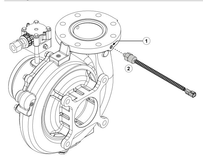
Use the illustration and instruction to install the pressure switch. The pressure switch is only required when operating the pump in auto-prime mode.
