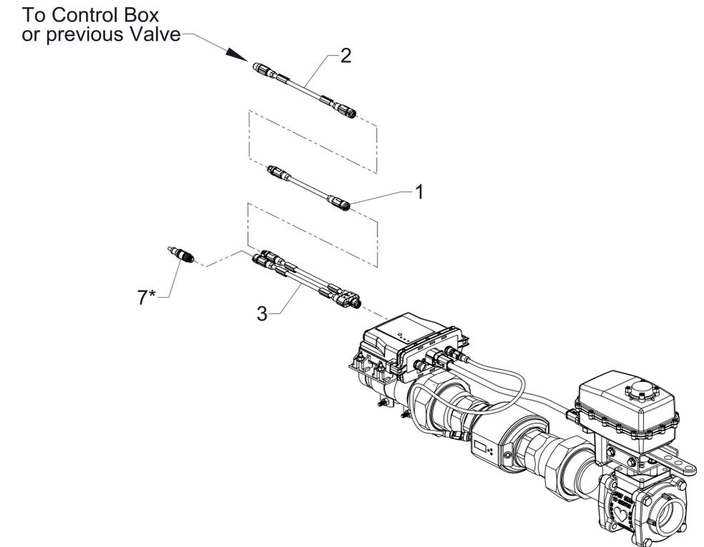
\* Note that resistor installed if valve is last valve in CAN string.
