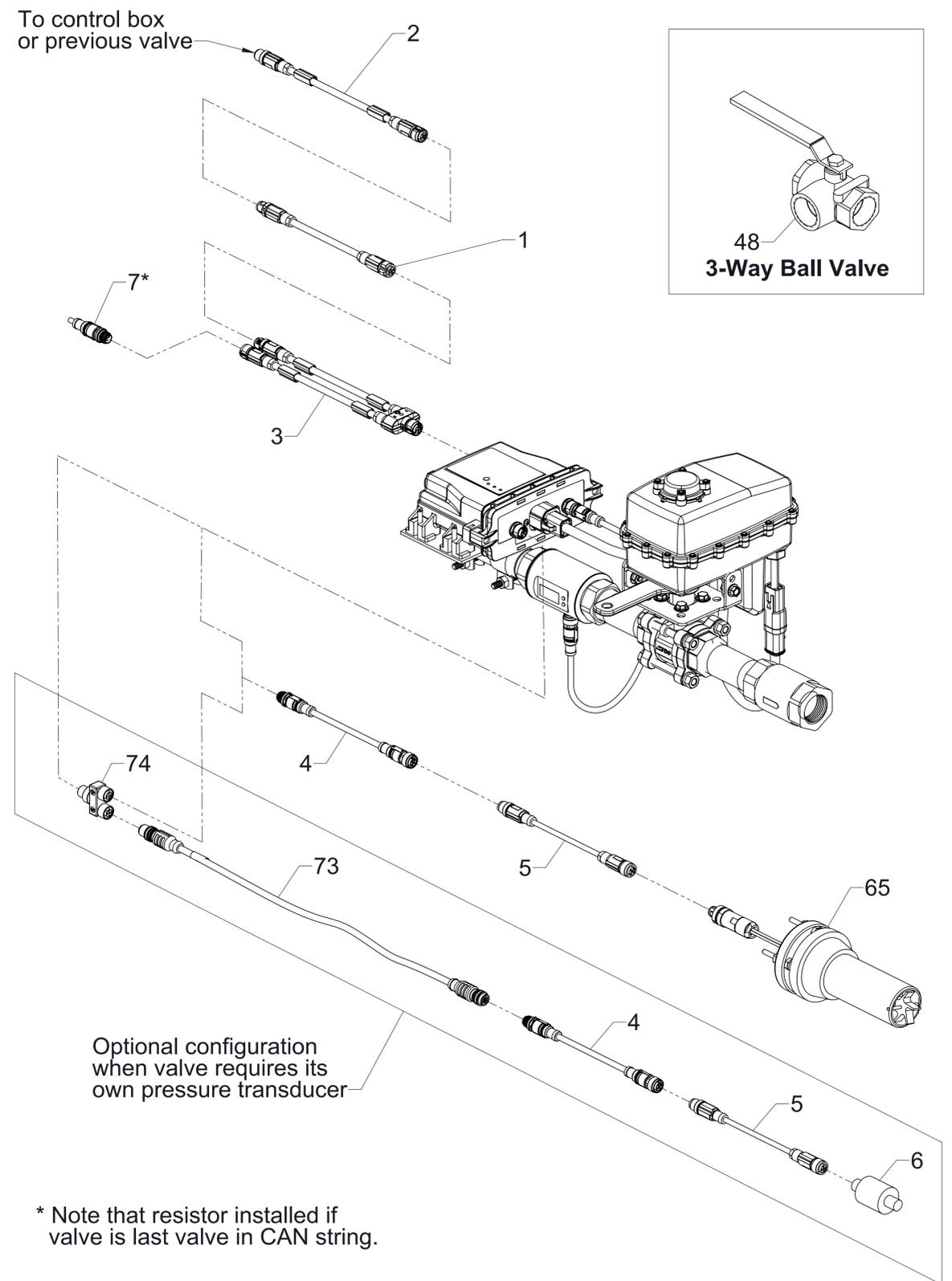
\* Note that resistor installed if valve is last valve in CAN string.
