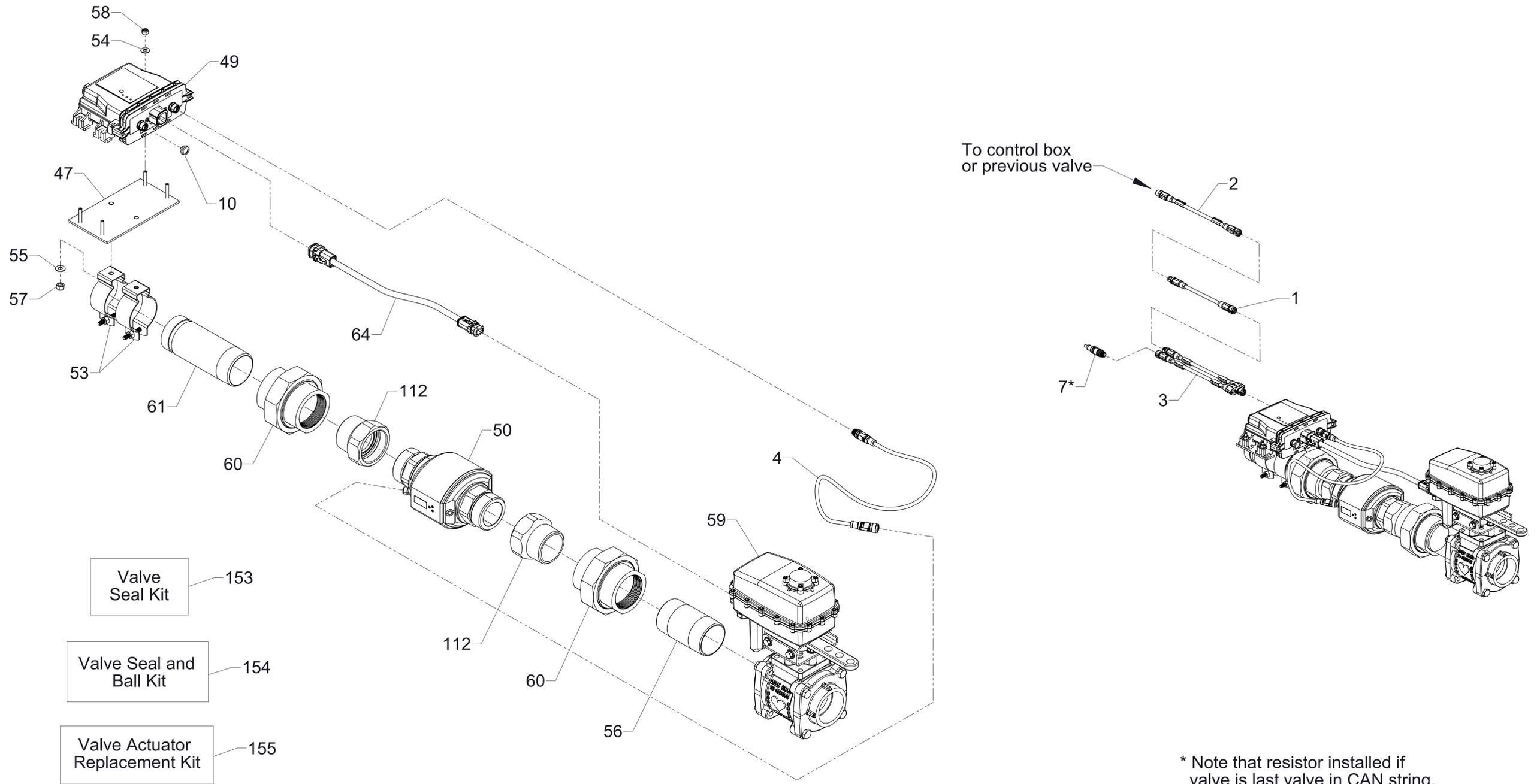
**2 in Low Flow By-Pass Valve Sub-Assembly**
