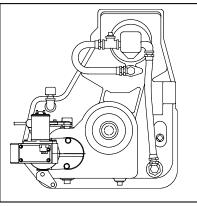
Electric shift on rear of pump transmission showing shift unit, indicating light switch and shift arm. When the shift arm is moved to the PUMP position it makes contact with the switch and activates the green ``PUMP ENGAGED" light circuit.
