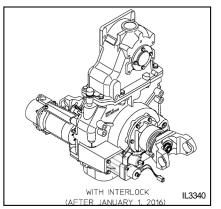
Pneumatic shift on the rear of pump transmission showing double acting air cylinder and indicating light switch. When the rod of the air cylinder is in the IN position, 1/2" exposed, the transmission is in the ROAD position. When the rod is in the OUT position, 1-1/2" exposed, the transmission is in the PUMP position and a switch is closed for activating the circuit for the green "PUMP ENGAGED" light on the in-cab panel plate.
