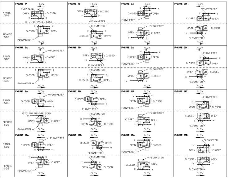
KEY: Y INDICATES A Ø.500/12.7 HOLE FORE RIGID ROD CONNECTIONS X INDICATES PROVISION FOR UNIVERSAL JOINT CONNECTION
