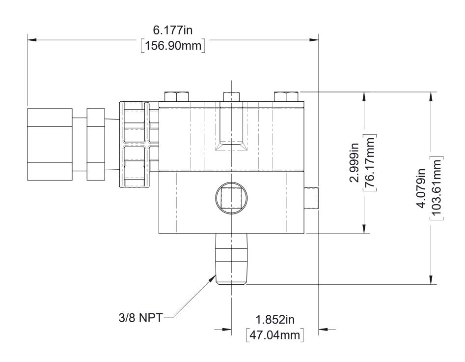
Dimensions of Valves Mounted by the OEM (Shipped Loose by Waterous)
