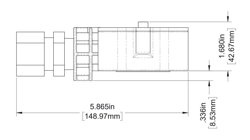
Dimensions of Pump Mounted Valves (Mounted by Waterous)
