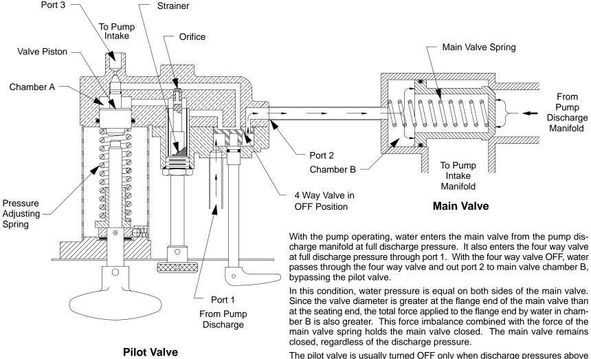
300 psi are required, or if higher pressures are desired without the necessity of disturbing the pilot valve setting.
