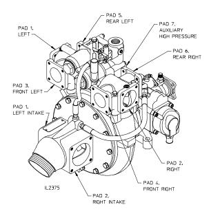
**Intake Adapter and Discharge Manifold Pads**
