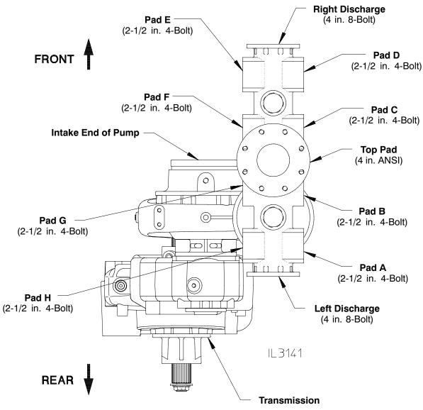
Note: Left and Right are Defined as Viewed From the Side of the Pump with the Transmission on Your Left and the Intake on Your Right.
