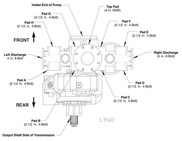
Note: Left and Right are Defined as Viewed From the Output Shaft Side of the Transmission.
