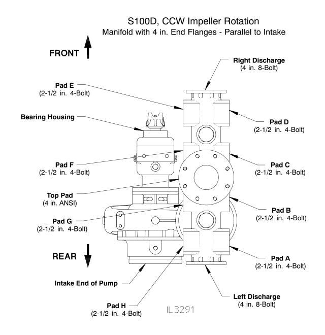
Note: Left and Right are Defined as Viewed From the Side of the Pump with the Intake on Your Left and the Bearing Housing on Your Right.
