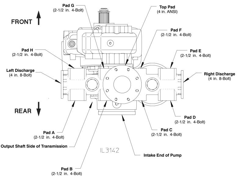
Note: Left and Right are Defined as Viewed From the Output Shaft Side of the Transmission.
