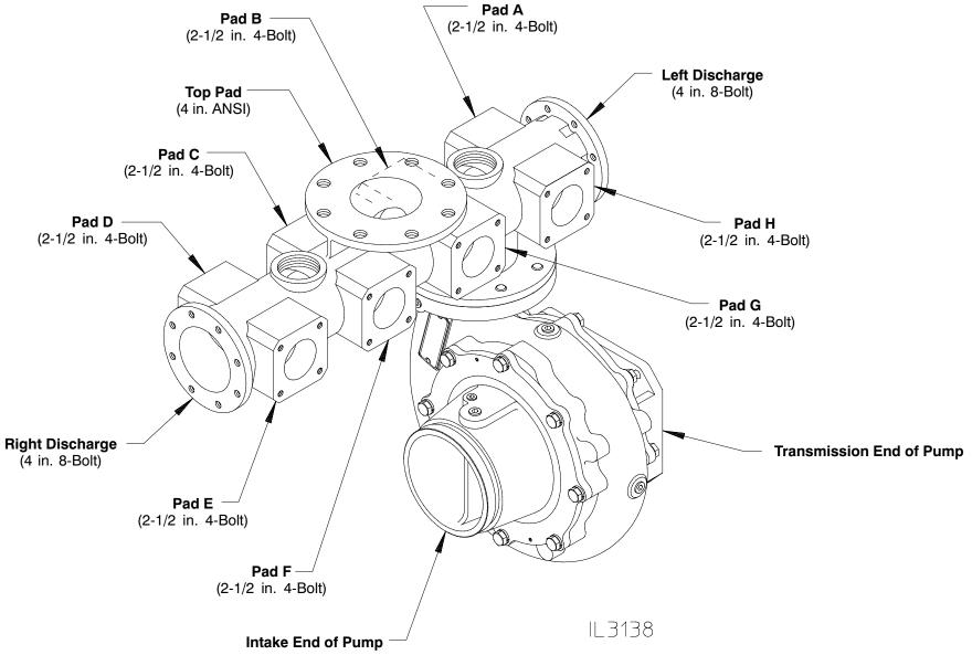
Note: Left and Right are Defined as Viewed From the Side of the Pump with the Transmission on Your Left and the Intake on Your Right.
