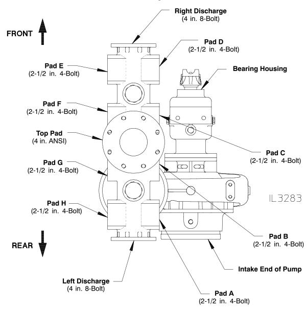
Note: Left and Right are Defined as Viewed From the Side of the Pump with the Intake on Your Left and the Bearing Housing on Your Right.
