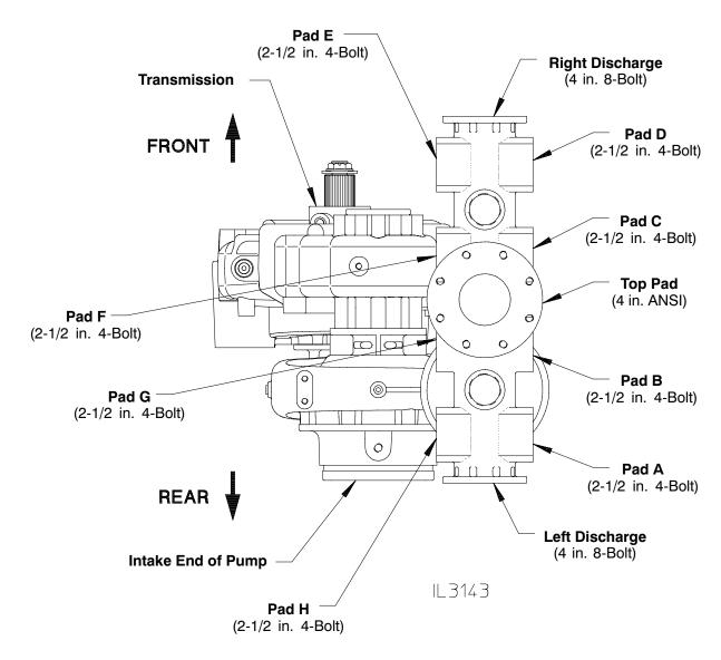
Note: Left and Right are Defined as Viewed From the Side of the Pump with the Intake on Your Left and the Transmission on Your Right.
