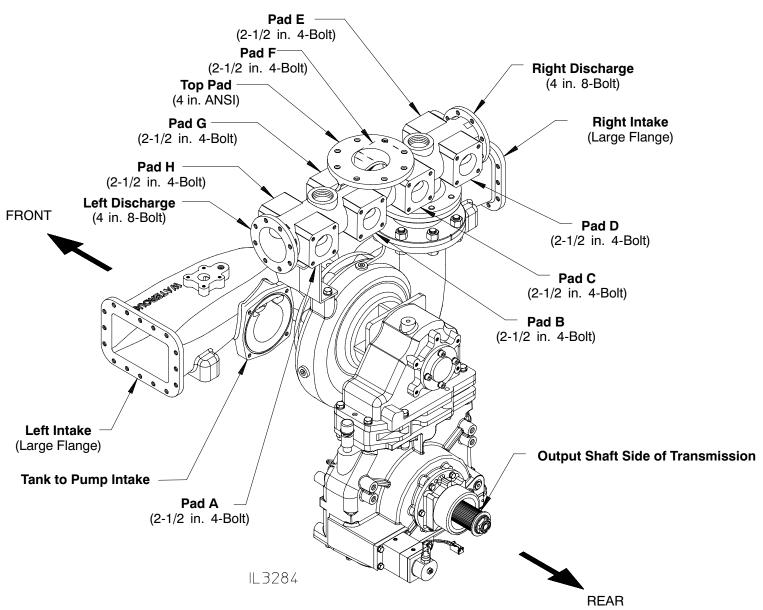
Note: Left and Right are Defined as Viewed From the Output Shaft Side of the Transmission.
