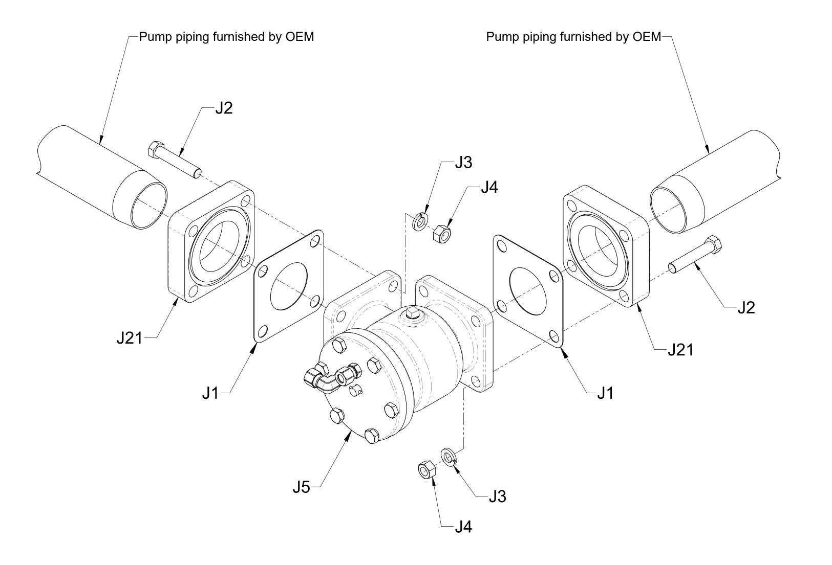
Flanges Sealed with Gaskets (Prior to September 28, 2009)
