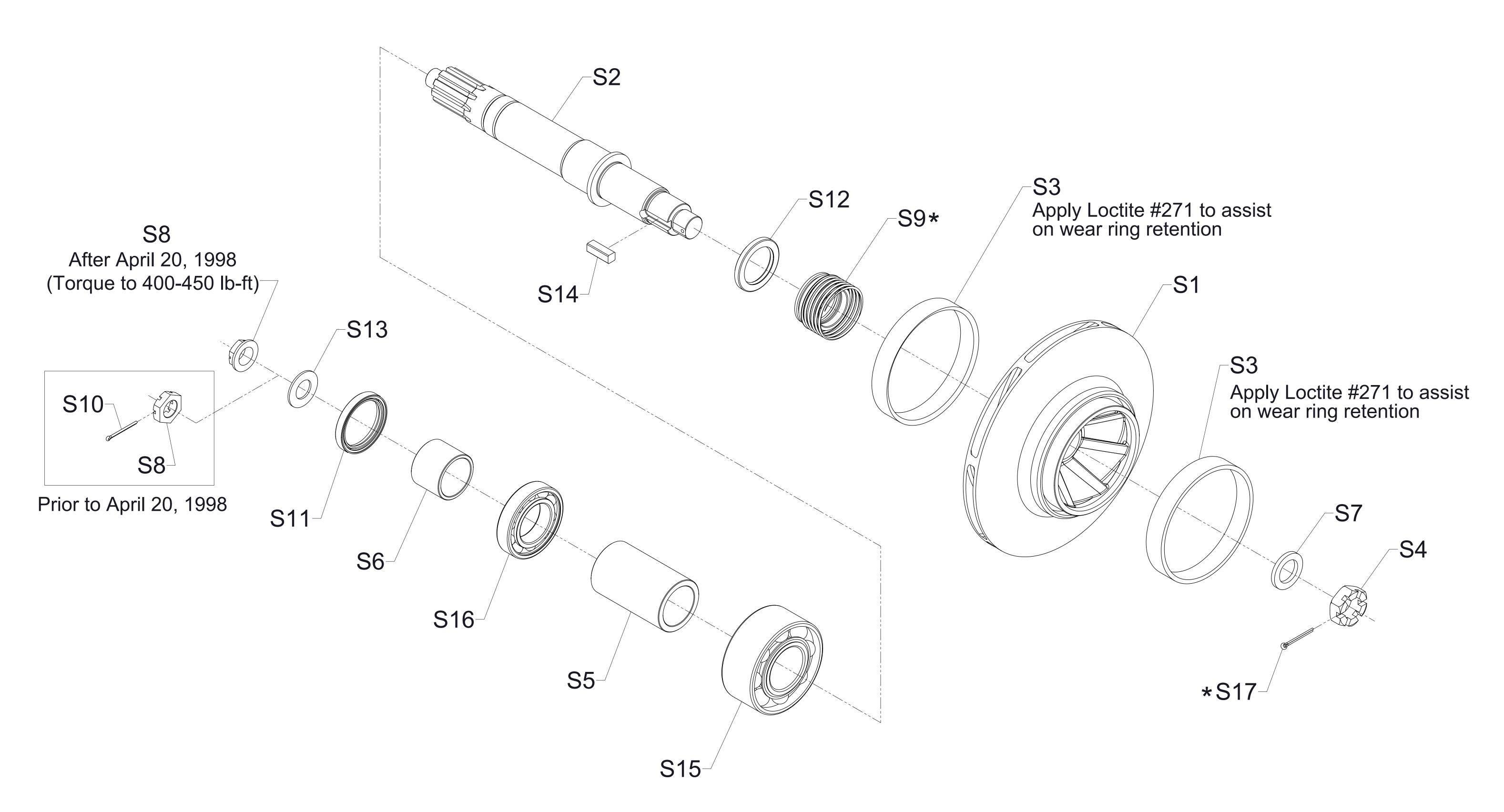
\* Included in Mechanical Seal repair Kit S9. Also includes O-ring B9 from Body Assembly
