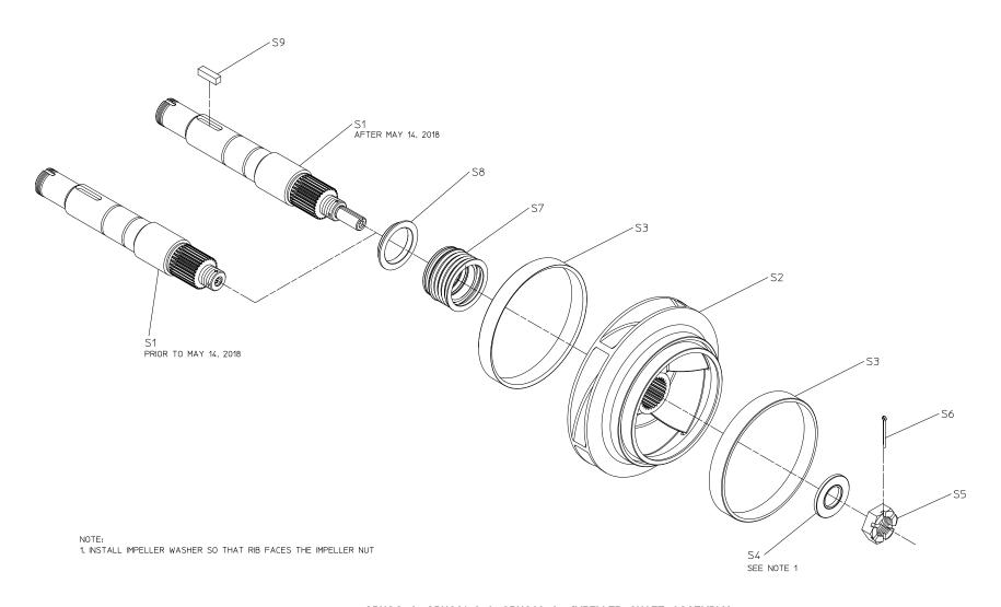
CRUQC-2, CRUC21-2 & CRUC23-2 IMPELLER SHAFT ASSEMBLY
