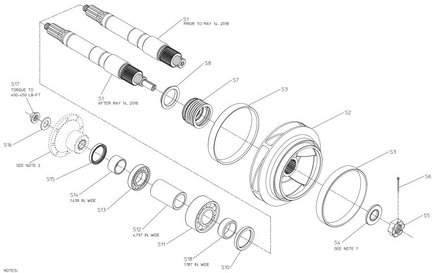
1. NSTALL IMPELLER WASHER SO THAT THE RIB FACES THE IMPELLER NUT. 2. COMPANION FLANGE OR END YOKE MAY NOT HAVE BEEN SUPPLIED BY WATEROUS.
