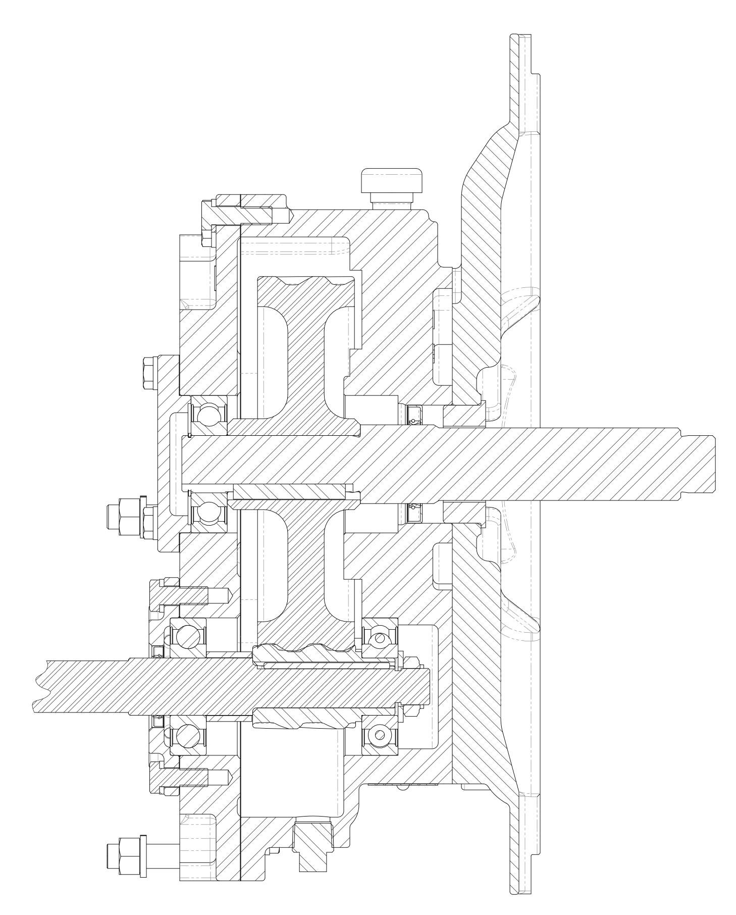
Transmission Assembly SAE - 3 Bellhousing Adapter
