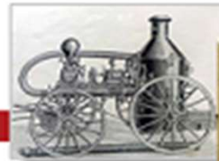
Waterous Steam-Driven Fire Engine
