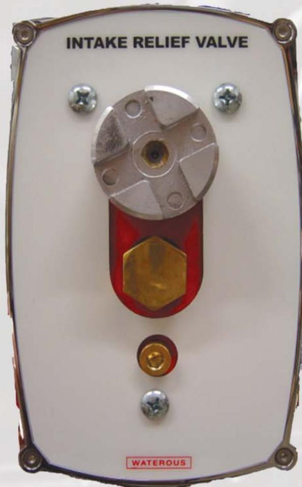
The Waterous Intake Relief Valve system is designed to act as a safety valve by "dumping" excess pressure from the inlet side of the pump. The Discharge Relief Valve provides sensitive pump control to protect firefighters from sudden pressure surges resulting from changes in discharge flows from the pump.
