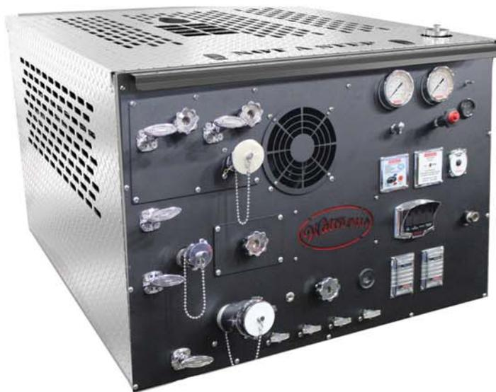
Our slide-in, portable modular compressed air foam 100-50-DS unit is designed and constructed to simultaneously discharge water, foam solution or compressed air foam, developing 80 GPM of water at 125 PSIG (300 L/min. @ 8.6 bar) and 40 CFM of air at 125 PSIG (1.13 m<sup>3</sup>/min @ 8.6 bar). The 100-50-DS also features compressed air for pneumatic tools and can pump water or air independently.
